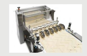
Motorized trim recovery for the maximum precision and cleaning
